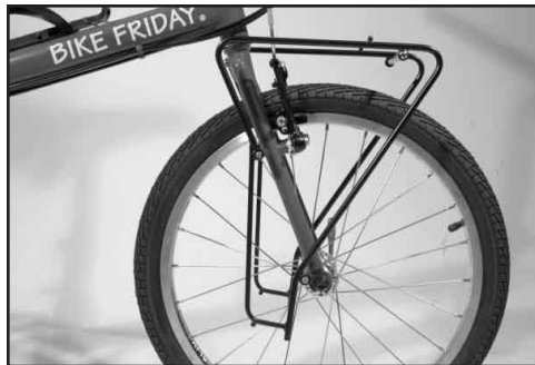
Fig. 6 Completed front rack.
